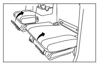
To access the storage compartments, lift the cushion on the bottom of the rear seats. This exposes the storage boxes under the seat.
